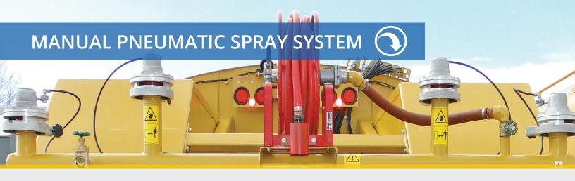
The manual pneumatic spray system is a simpler, cost-effective alternative to the electro-pneumatic spray system, and is available for use on any 24 volt truck with a reliable air supply. The manual pneumatic system can be configured for either an electric or hydraulic water cannon, and comes with a separate tractor air supply protection valve, air-pressure regulator, and manual shut-off valve.
